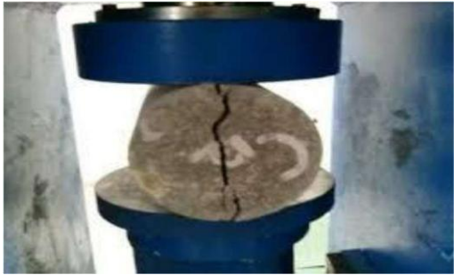
Fig .Split Tensile Strength of Cylinder
