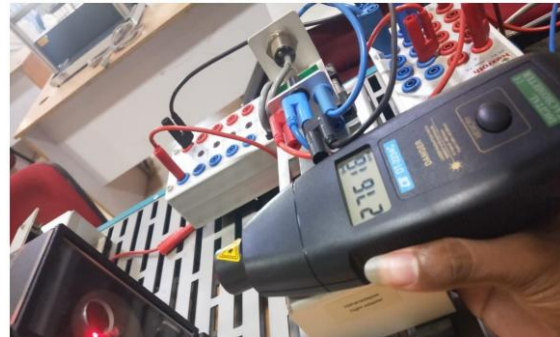
Figure 6: measure the speed of the motor in RPM
