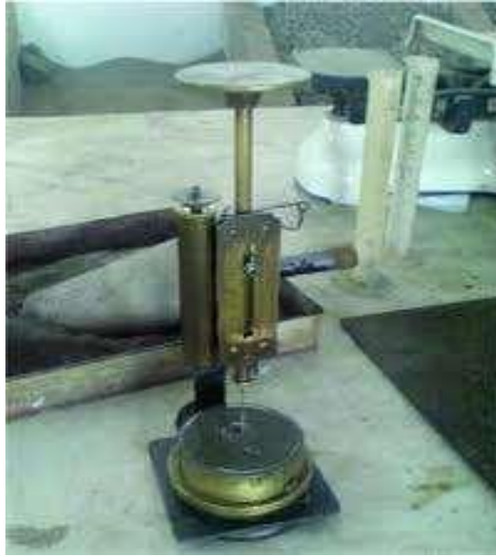
Fig5.2 Vicat Apparatus to find initial setting time
