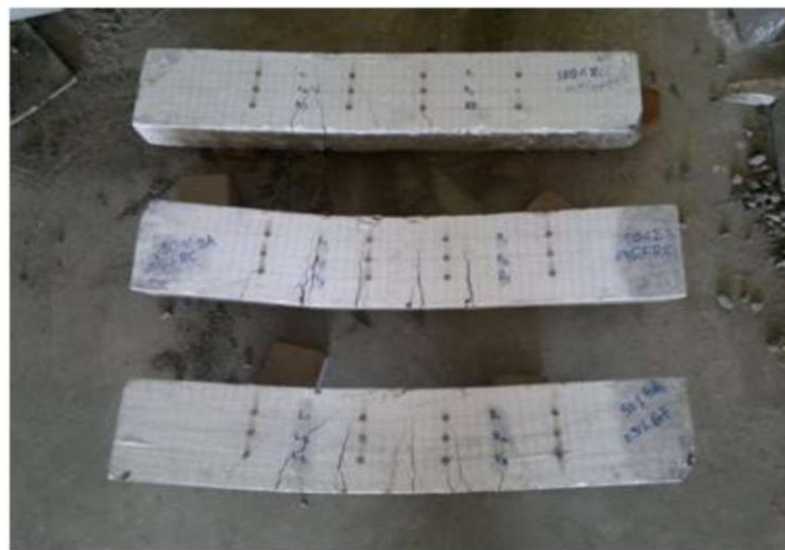
Flexural cracks in control beam and beam with BGC3 mix
