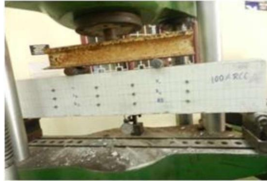
Fig 7.5 Flexural Beam Test
