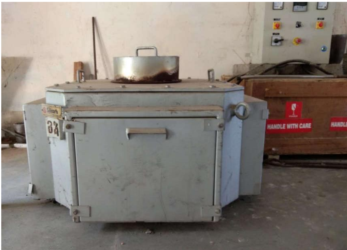
Fig.1 Elecrtric resistance furnace with controll unit.
